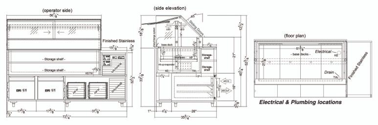
1. A 1 1/8" diameter drain is provided. The drain MUST be connected to a floor drain or storage container AT TIME OF INSTALLATION.
