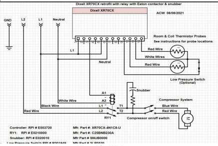
(wiring term. (3 Comp.) (1 Line), (5 line Jumper from 1) (6 Neutral) Two temperature probes See Note Below
